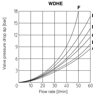
**8 OPERATING LIMITS** based on mineral oil ISO VG 46 at 50°C
