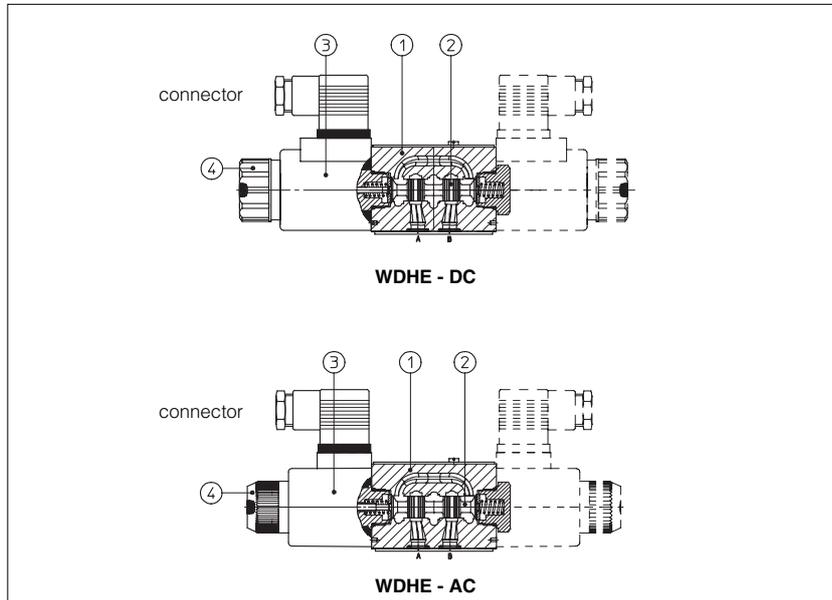
Spool type, direct operated solenoid valves available in three or four way configurations and with two or three spool positions, see section 2.
